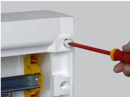
We recommend using a 6.5 mm flat screwdriver to open and close the XL³ 125 cabinets, and also for positioning the faceplates with a ¼ turn, for which 1 Nm tightening torque is sufficient.
